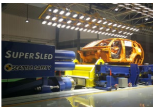
FITP’s accelerating sled testing system used for head-on collision tests. IID Tsukuba Technical Center Source: The company’s website
